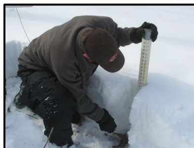
Obtaining snow depth and core sample
