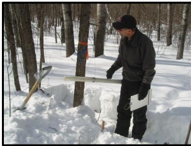
Establish base weight of empty sampling tube
